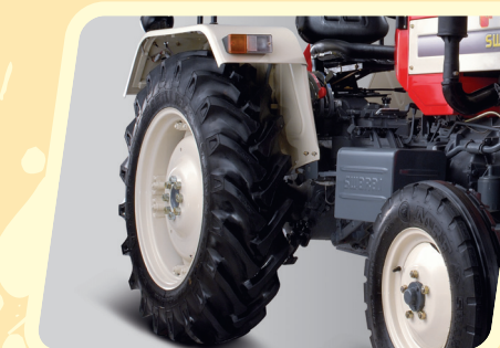
345.44 X 711.2 mm (13.6 x 28) rear tyre For strong hold in tillage and other work
