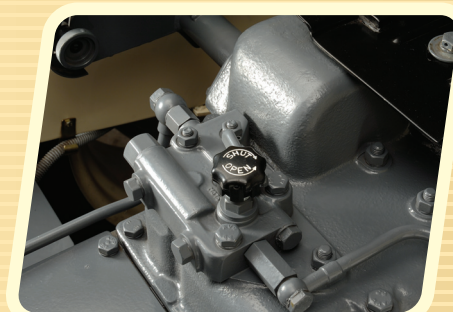
Better control valve Helps in maintaining uniform depth in sowing and pushes the sandy mud to make proper level.
