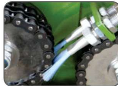
Centralised self lubrication system with cleaning brush
