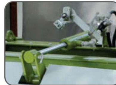
Hydraulic bale eject system
